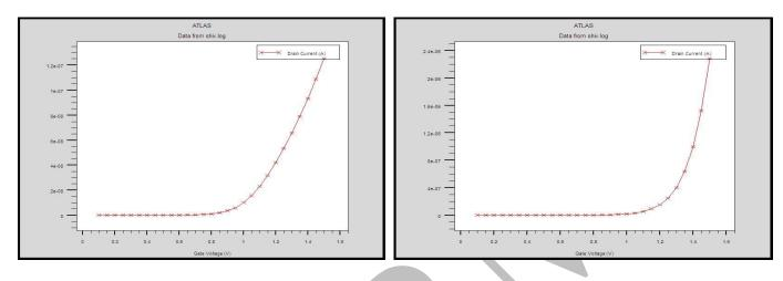
(a) (b)Figure 5:- Id-Vgs Characteristics of Single Gate FDSOI n-MOSFET at (a) Vds=0,1v (b) Vds=1.5vrespectively.
