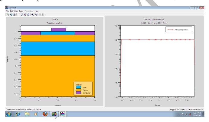
Figure 8:- Net Doping Effect of Single Gate Fully Depleted SOI n-MOSFET Channel Length of 100nm
