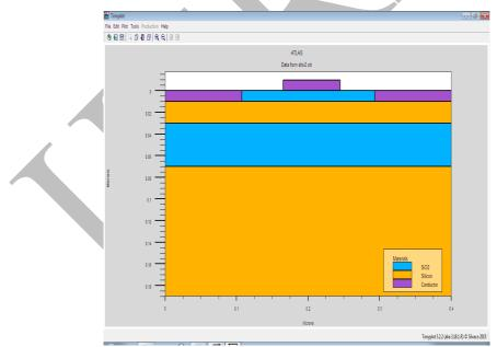
Figure 4:- Device Structure of the Single Gate FDSOI n-MOSFET with effective channel length 0.1um channel doping is 1E18cm<sup>-3</sup> and drain and source doping concentration is 1E20cm<sup>-3</sup>gate oxide thickness is 0.01um
